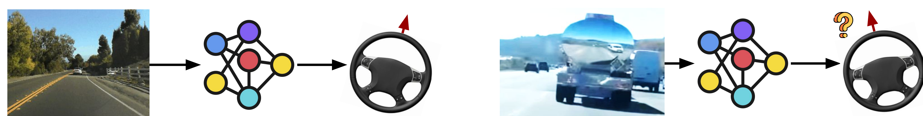
Figure 1. ML model problem due to simple association of input with output. (a) An ML model trained with pairs of images from a front-facing camera and steering angle. The ML model works well as long as the input has a similar distribution to training datasets. (b) Even a successful model will show unexpected behaviors when the input data has a significant distributional shift (a reflected road image on the car in front) from the training datasets.
